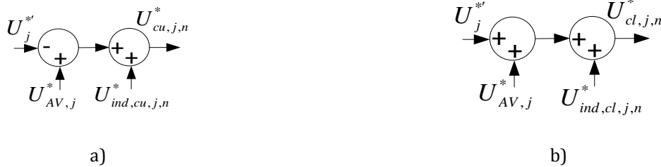
Figure 6-12 Reference signals for the n^{th} SM in the j^{th} phase in the a) upper arm and b) lower arm.
