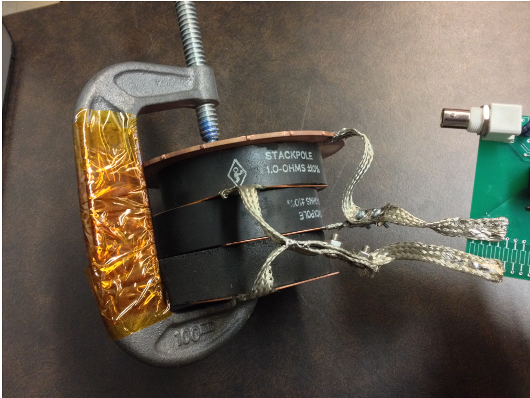
Figure 3.6: Carbon composition resistors used for low impedance loads. The configuration here is measured to be 0.3\ \Omega . The C-clamp is isolated from the top plate by multiple layers of kapton tape.
